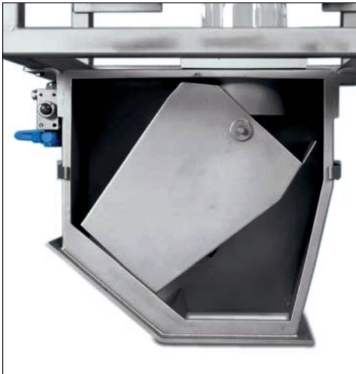
Separation unit with opened cleaning flap.
