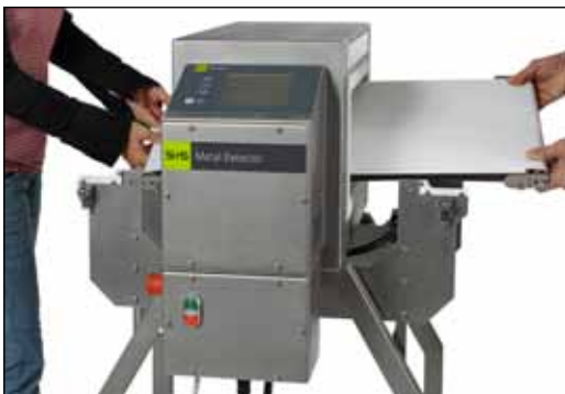
Belt run adjustment is not necessary with the ECOLINE-D metal detection system because of the profile on the back-side
